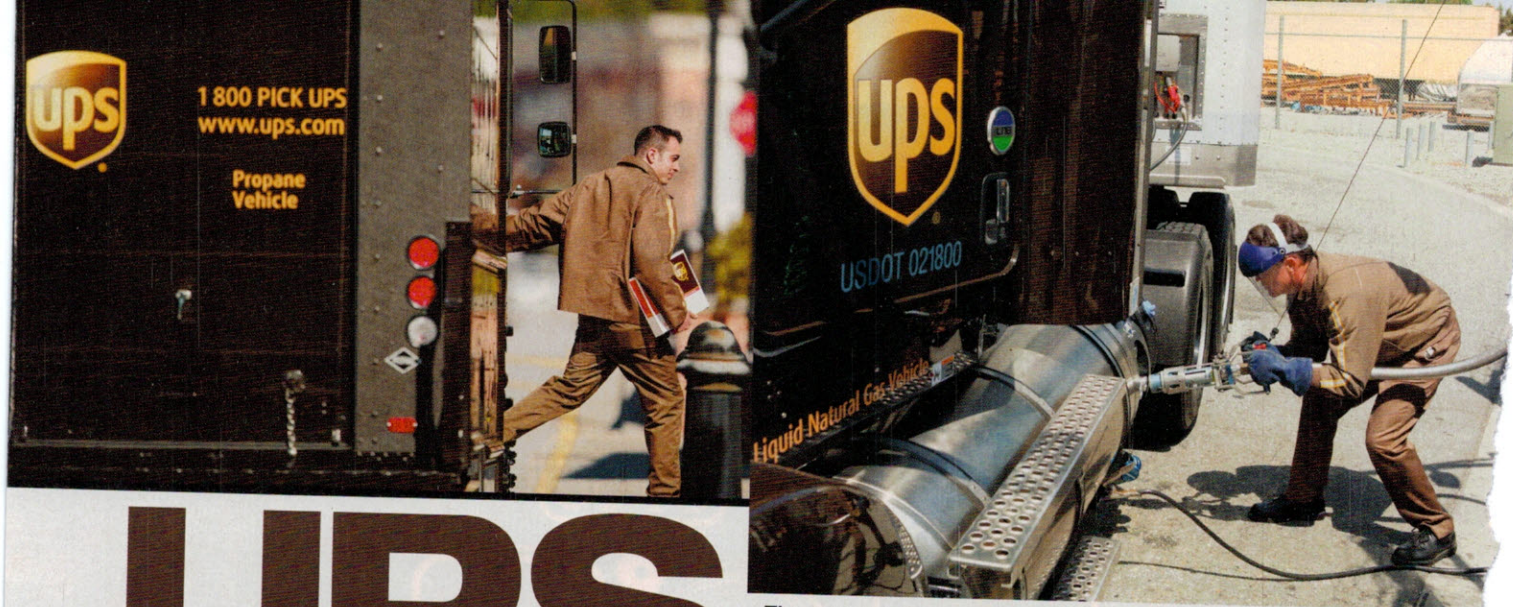
The parcel delivery company utilizes multiple alternative fuels in its vehicle fleet, including propane autogas (left image) and natural gas (above).
